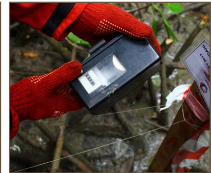
Observations and assessment of the community structure are done using 25 x 25 meters (m) plots delineated using tape, cotton string, wooden pickets (left onsite for future surveys to allow comparisons), and hand-held laser measurements.
